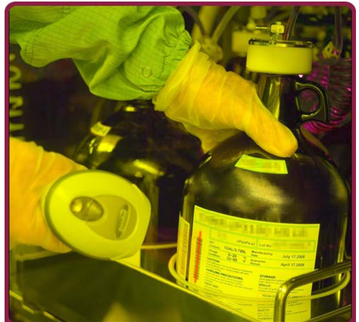
Figure 1. The manufacturer's bar code and other information is collected and evaluated during a resist change.
